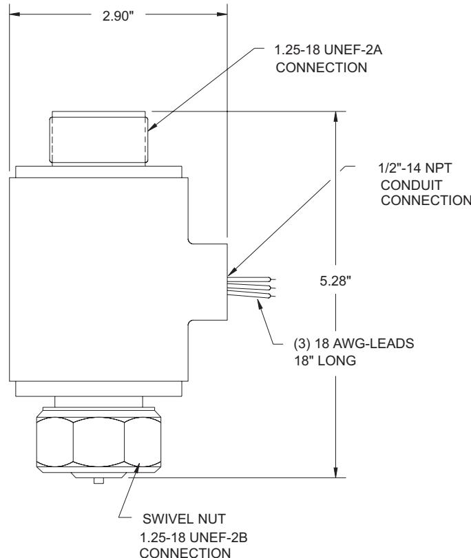
**Note:** This control head is polarized. Improper wiring will result in operational failure of this device.
