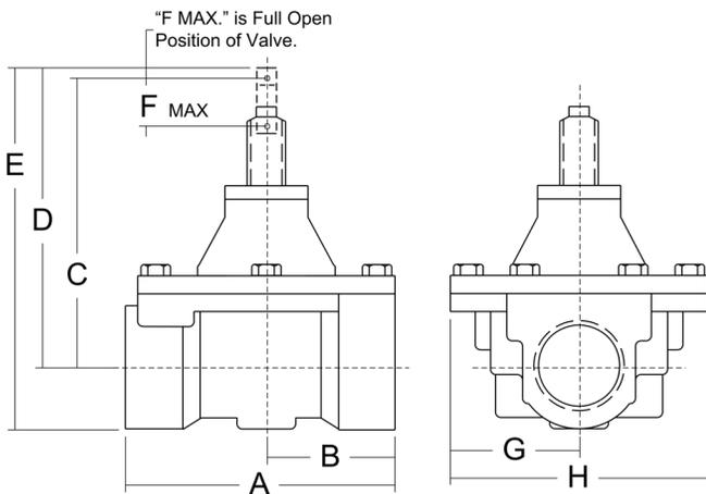
Figure 3. Dimensions of the Mechanical Gas Valve
