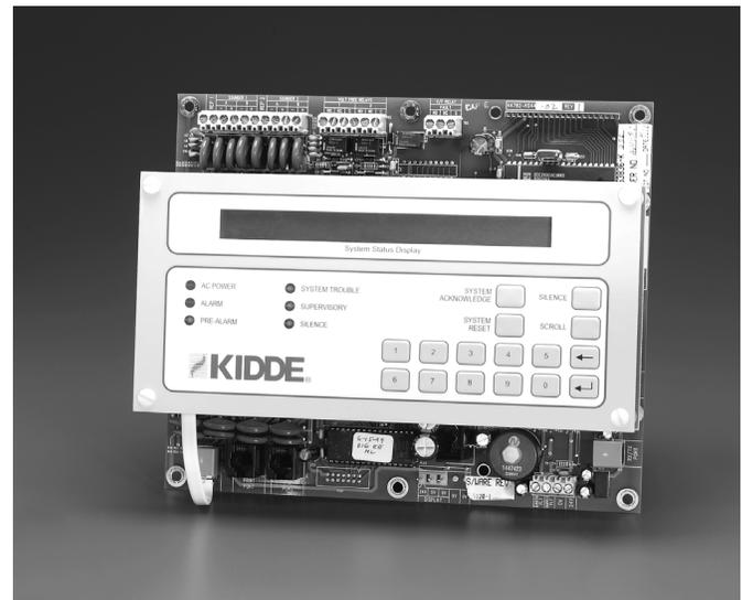
Two individually-programmable notification appliance circuits (MP1 and MP2) provide up to 2.0 Amps of 24 Vdc power for horns, bells and strobes. The MP1 output can be optionally programmed for releasing solenoid type suppression equipment (agent and sprinkler).
