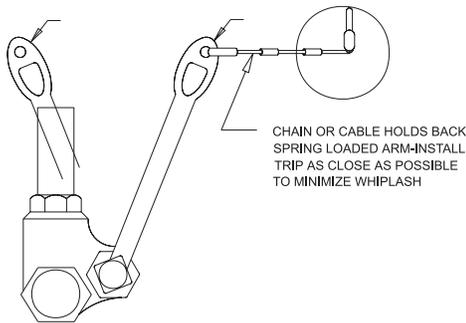
SPRING LOADED LIQUID OR GAS SHUTOFF VALVE
