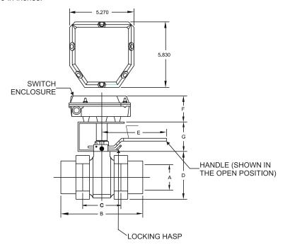
MATERIALS BODY: CARBON STEEL WITH BALL AND STEM: 316 STAINLESS SEATS AND SEALS: TEFLON
