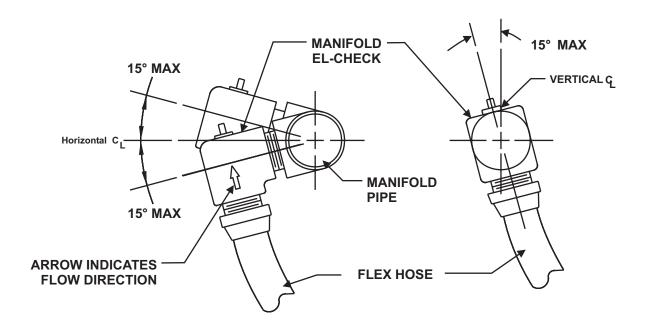
**Notes:** Install El-Checks so that the arrow is in the direction as indicated.
