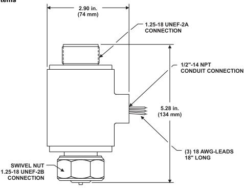
**Note:** This control head is polarized. Improper wiring will result in operational failure of this device.
