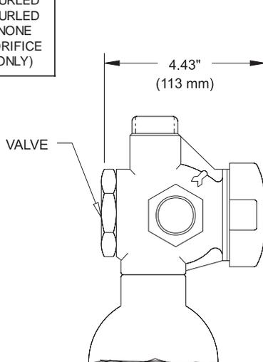
INLET AND OUTLET MAY BE REDUCED WITH BUSHING OR BELL REDUCER AND NIPPLE TO 1/2" NPT IF NECESSARY.
