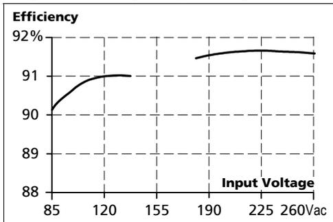
Fig. 9-4 Losses vs. input voltage, 48V, 5A
