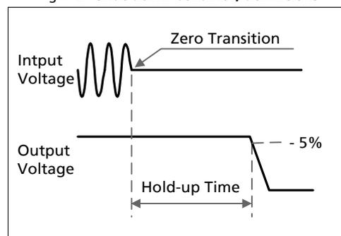
Note: At no load, the hold-up time can be up to several seconds. The green DC-ok lamp is on during this time.
