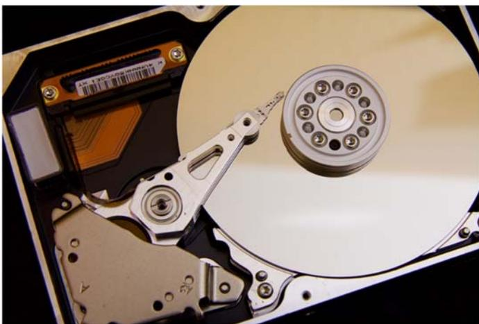
on the platters by the write head which changes the magnetization of individual data cells. The cells are organized in tracks that encircle the disk. There are about 10,000 parallel tracks in each millimeter of the platter. The “read” operation is done as the read head passes over the data cells; the magnetization of the data cells induces a current in the read head which is decoded by the HDD circuitry and converted to binary values for interpretation by the operating system and software.
